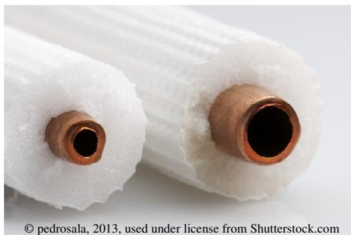
For automatic circulating hot water systems, piping shall be insulated with 1 inch of insulation having a conductivity not exceeding 0.27 Btu per inch/H x ft<sup>2</sup> x F°. This is equal to an R-3.7 per inch thickness.
